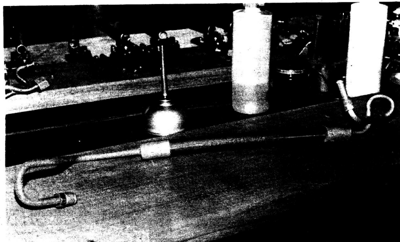
HERE IS AN example of a finished bending fixture, which is ready to go to the factory. The model bending fixtures take anywhere from three to five weeks to complete. Each bend in the fixture is done on a different mechanical arm.
