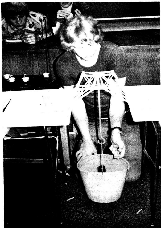
CAUTION is the word as Williams adds more weight and Darrell Hudson anxiously peers over his shoulder. Note that the bucket has begun to buckle and that he stacked many of the weights on top of each other.
