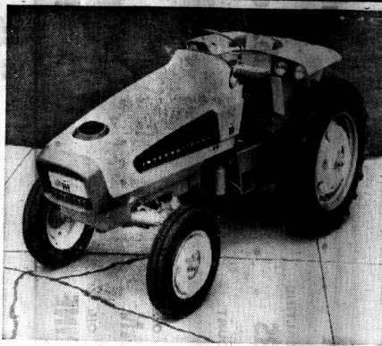
International Harvester Company's experimental tractor has a gas turbine engine paired with a hydrostatic transmission. Skin, or body, sections are molded fiberglass.
