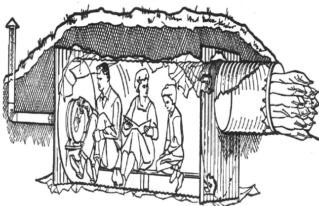
PRE-FAB corrugated steel culvert fallout shelter, radiation exposure of its occupants, is included for three persons can be bought for about $150, in the "Family Shelter Designs" booklet now plus delivery and installation. The shelter, which at state and local civil defense offices for public would cut to 1/500th the amount of outside fallout distribution. It is available without charge.
