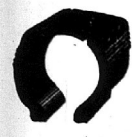
Section of smooth tire which is liable to punctures, blowouts and skidding.
